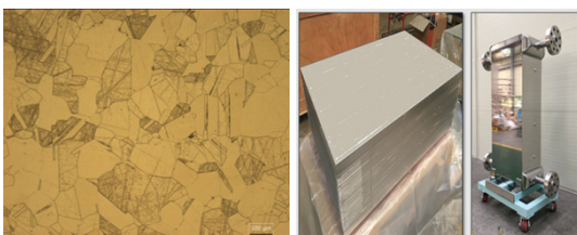
Fig. 4. Surface after diffusion bonding and PCHE
