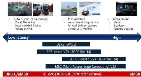
Fig. 1 Positioning by communication technology by self-driving function/service(Sources: Huawei)
