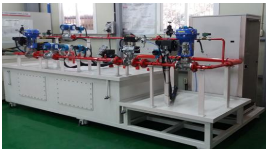
Fig. 1 Experimental setup for C_v measurement
