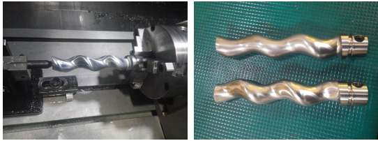
(b) After finishing process and machining result by ball end mill tool
