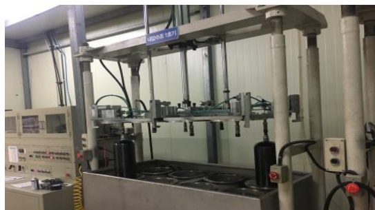
Fig. 8 Internal pressure test of ANG fuel tank
