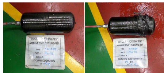
Fig. 9 ANG fuel tank before and after burst test
