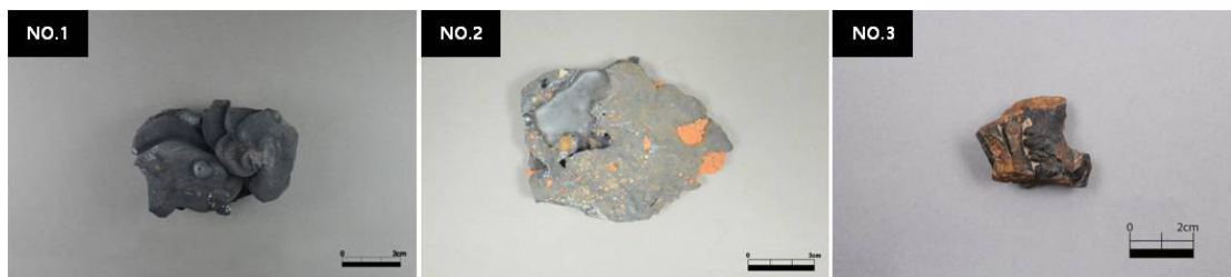
Figure 1. Slag samples. (Left) Smelting processes on iron sands collected from Pohang, (Middle) Smelting processes on iron sands collected from Gyeongju, (Right) Excavated from copper smelting site at Wanju.
