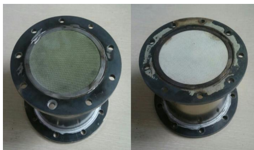
Fig. 3. The photograph of the canning zeolite based Cu-ZSM-5 catalysts and Cu-CHA catalysts
