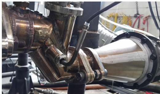
Fig. 1. The photograph of the exhaust layout installation in engine test bench
