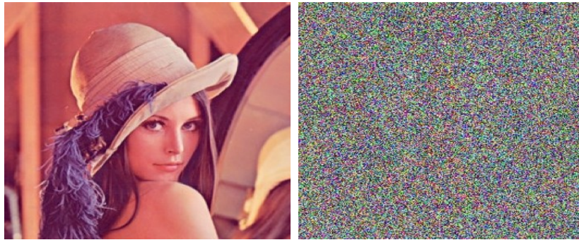
Fig. 5. The decrypted Lena image with correct keys (left) and with a small noise added to Key_c and Key_t (right).
