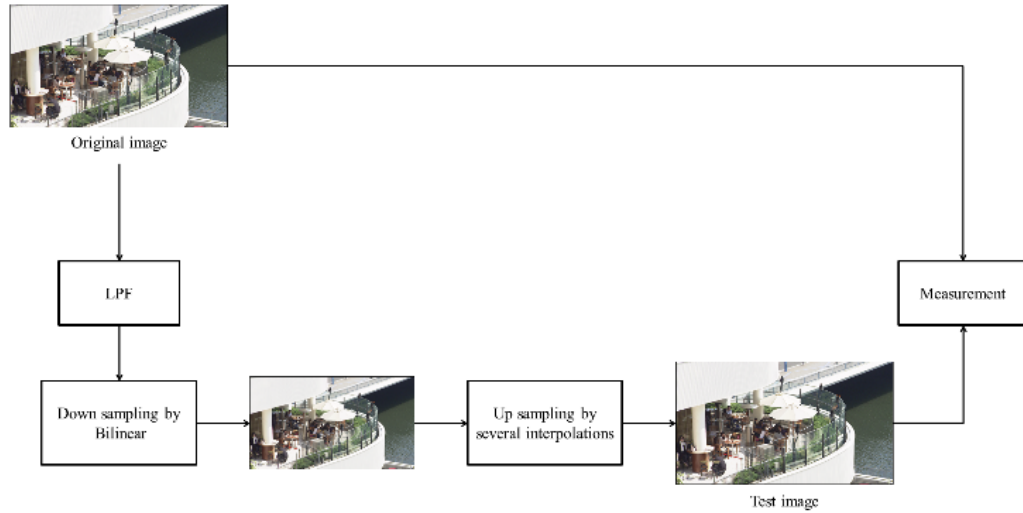
Fig. 3. Block diagram of PSNR and SSIM measurement
