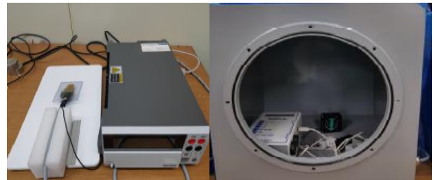
Figure 3. Thermal conductivity measuring instrument and radon gas measurement chamber
