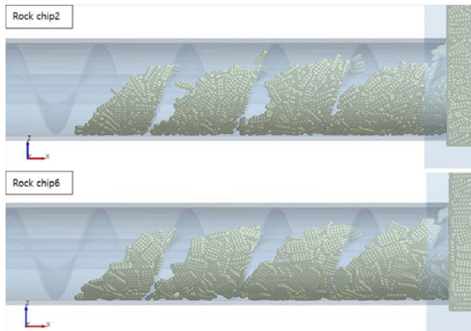
Fig. 4. Screw conveyor DEM simulation for discharge of rock chip 2 and 6 after 24 seconds
