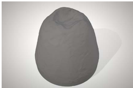
Fig. 9. 3D Image example of slim type conical pick (34th pick on the left drum)
