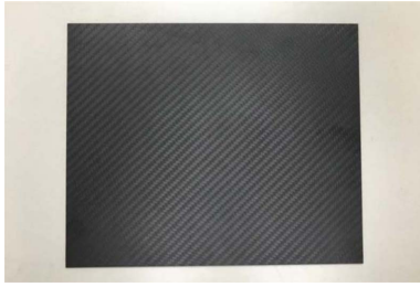
Fig. 3. Carbon fiber composite plate fabricated with RFI process
