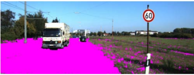
Fig. 8. Result of the proposed drivable area detection method with vegetation area removal.
