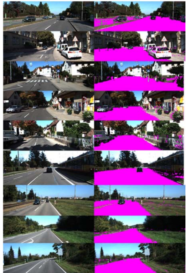
Fig. 12. Results of the proposed drivable area detection method.
