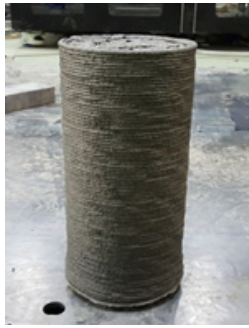
(a) Cylinder for Compressive Strength
