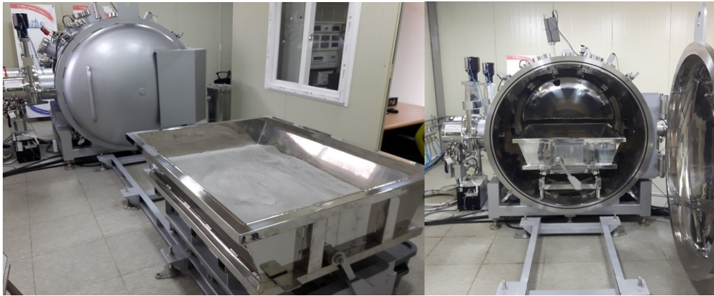
Fig. 2. Pilot Dusty Thermal Vacuum Chamber (DTVC)
