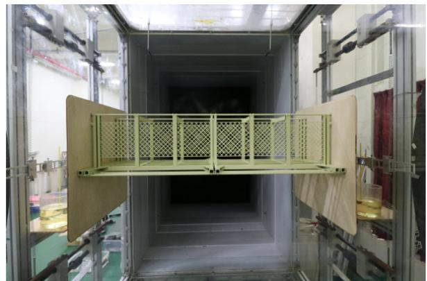
Fig. 13. Bridge Section Model
