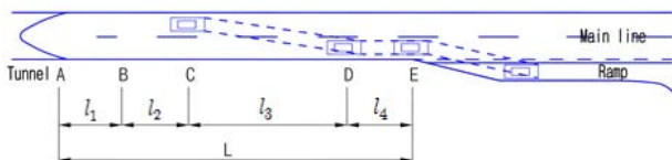
Fig. 12. Movement Path of the Vehicle Lane Change After Improvement
