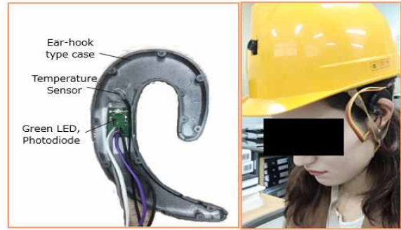
Fig. 2. Structure of Ear-probe and wearing the safety helmet
