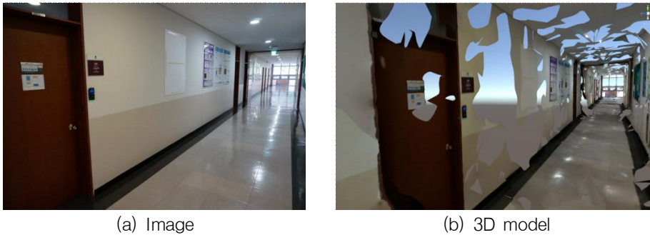
(a) Image (b) 3D model FIGURE 7. 3D models from photos with sparse keypoints
