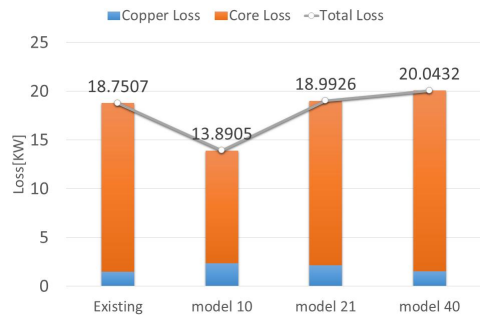
Fig. 4. Loss comparison by a Coil Cross-Section
