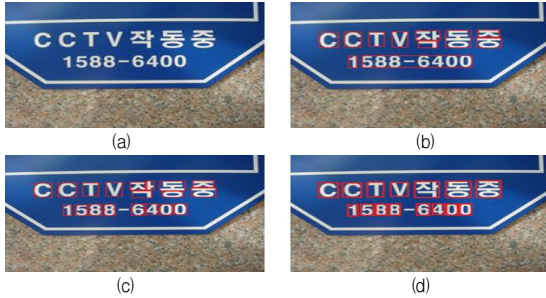
Fig. 15. Comparison of experiment results ③ (a) Original image (b) K-means detection (c) MSER detection (d) Proposed method
