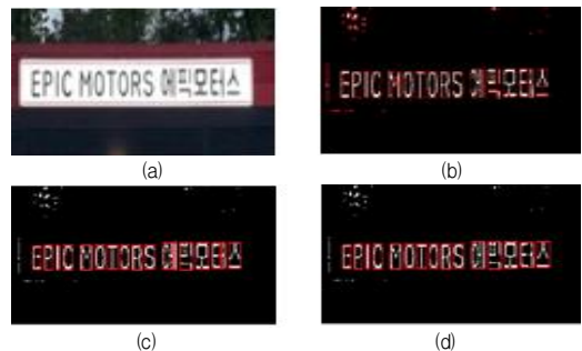
Fig. 12. Image of experiment result ③ (a) Original image (b) MSER detection result (c) Cumulative histogram detection result (d) Proposed method
