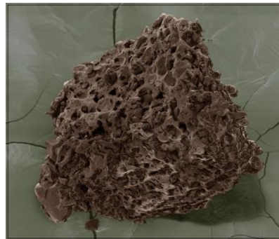
Fig. 1. Porous structure of coffee grounds by using quanta 3D microscope
