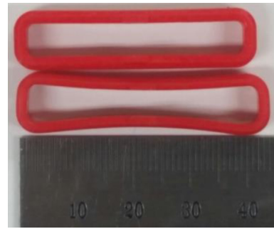
Fig. 11. Seal samples before and after aging tests at 120°C for 500 hours.
