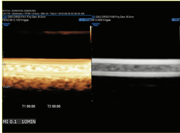
Fig. 8. Show increasing visual far wall artifact (arrow) with increasing concentration of micro bubbles within the flow phantom. (A) Contrast-enhanced image is on the left and (B) B-mode reference is on the right.
