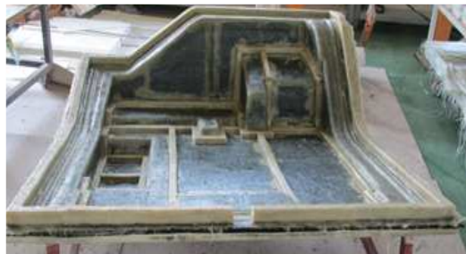
Fig. 12 Lamination of Glass Composite for Mould Manufacturing
