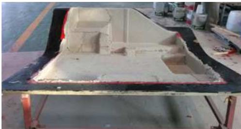
Fig. 14 Flax Fiber Lamination of Tank Lower Part
