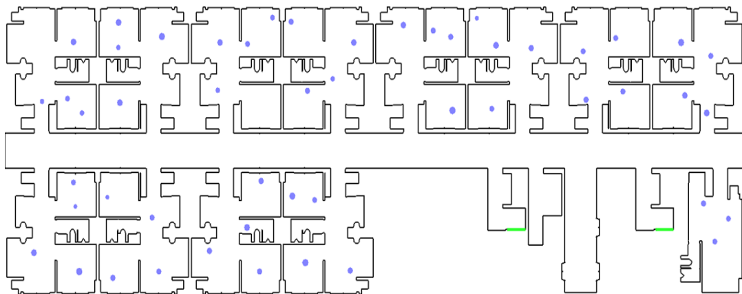
Figure 2. Geometry and Agent Location Setup for Evacuation Simulation using Pathfinder
