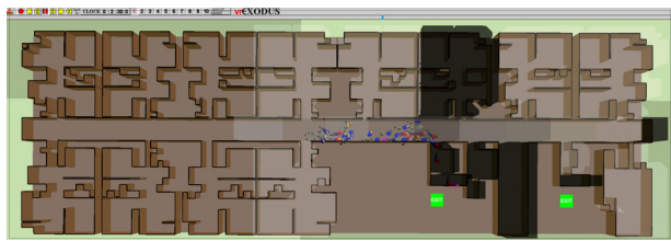
Figure 5. A Scene of Fire and Evacuation Coupling Simulation (T=150 s, 18 agents finished).
