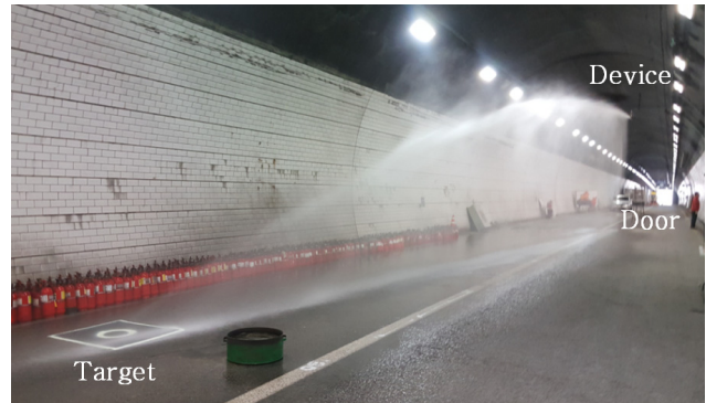
Figure 4. Water jet experiments in road tunnel.
