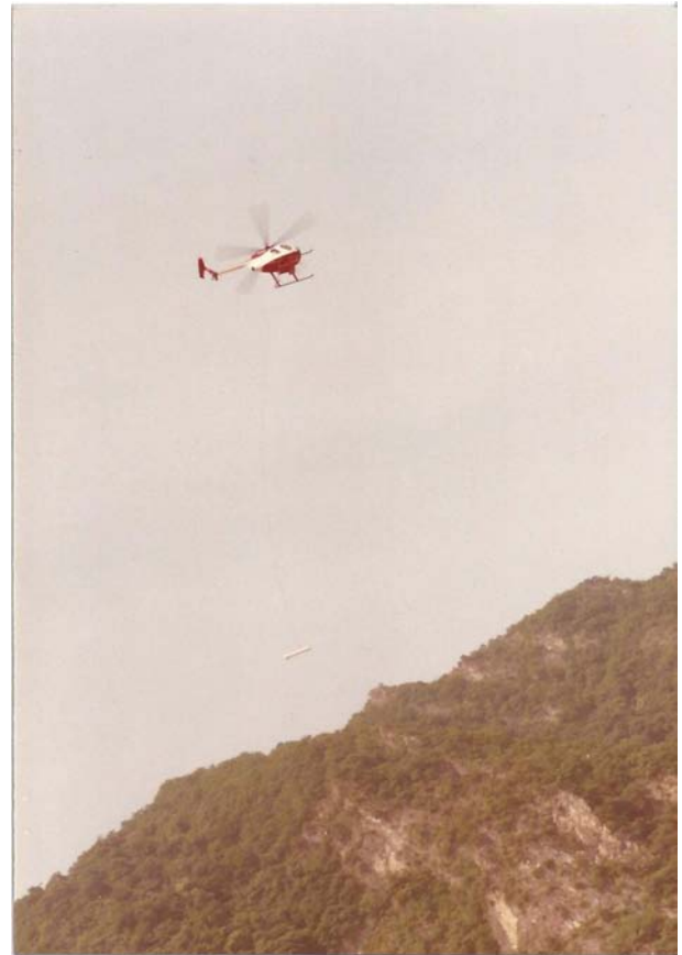
Fig. 1. Towed-bird type KIGAM airborne magnetic survey system since 1982.
