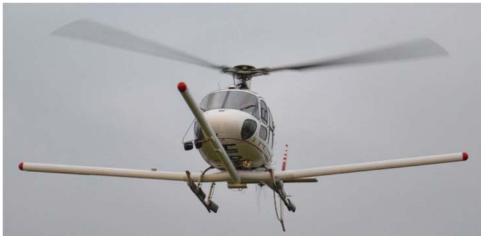
Fig. 2. 3-axis boom type KIGAM airborne magnetic survey system since 2013.
