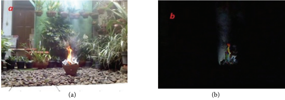
Fig. 2. An original frame containing fire (a) and the frame containing fire after background subtraction (b).
