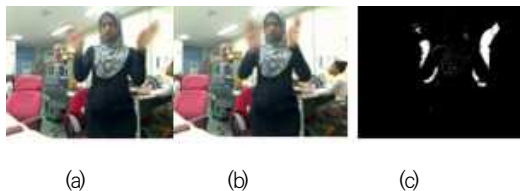
Fig. 3. Motion segmentation. (a) Previous frame. (b) Current frame. (c) Motion segmentation.
