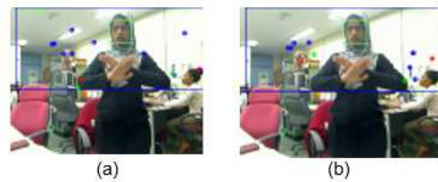
Fig. 5. Left and right arm gestures tracking within search area along face. (a) N-tracking points. (b) Average N-tracking points.
