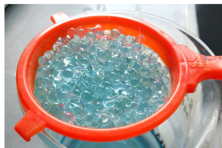
Fig. 1. Photograph of alginate beads used as a carrier for cell immobilisation of the potential SOB isolates.
