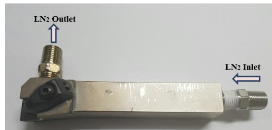
(b) Indirect cooling tool holder
