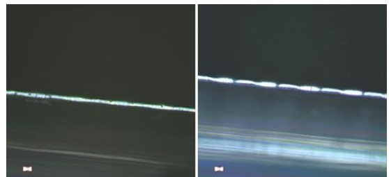
Fig. 12 Flank wear of zigzag type (K40UF) Left(Tetrabond), Right(Tisinis)
