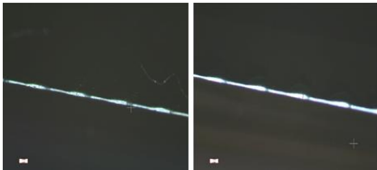
Fig. 5 Flank wear of normal type (K40UF) Left(Tetrabond), Right(Tisinis)
