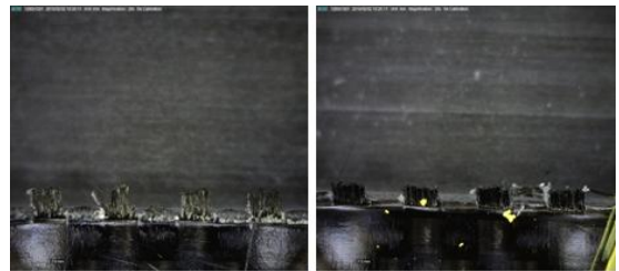
Fig. 11 Surface of CFRP (K55SF) Left(Tetrabond), Right(Tisinis)
