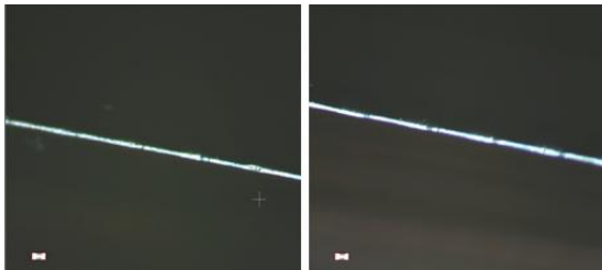
Fig. 6 Flank wear of normal type (K6UF) Left(Tetrabond), Right(Tisinis)
