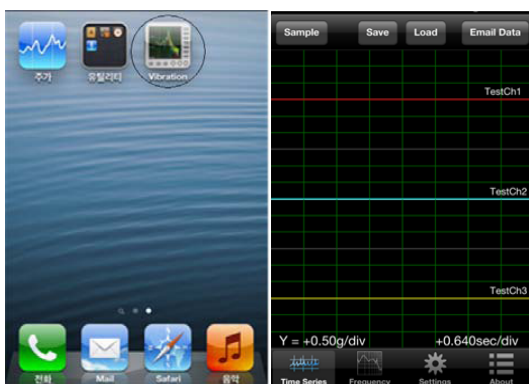
(a) Vibration measuring instrument - App (b) Vibration measuring instrument - Main view <Fig. 3> Vibration of iOS app (Vibration app ver. 2.01) 8)
