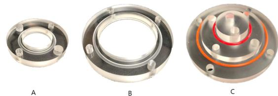
Fig. 2. Separation form of phantom frame(A: endocardium fixed frame, B: epicardium fixed frame, C: base frame and rubber packing ring)
