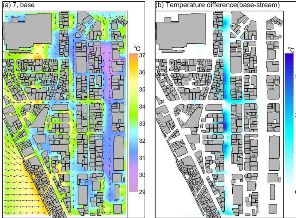
Fig. 6. Overall temperature distribution of 7, base case(a) and temperature difference between base and stream case(b).
