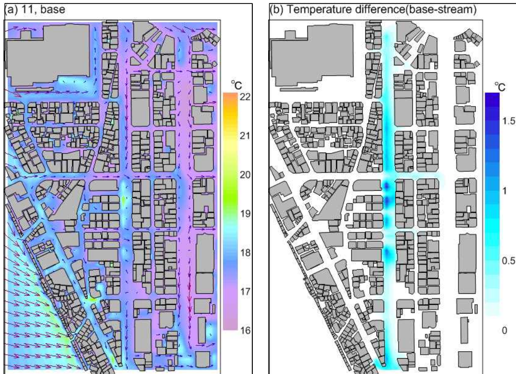
Fig. 5. Overall temperature distribution of 11, base case(a) and temperature difference between base and stream case(b).
