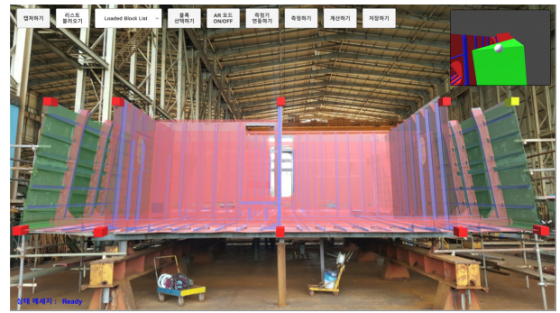
Fig. 10 Result of matching between actual block and 3D CAD model and measurement points. Detailed visualization window displayed on the screen by selecting measurement point(top right)
