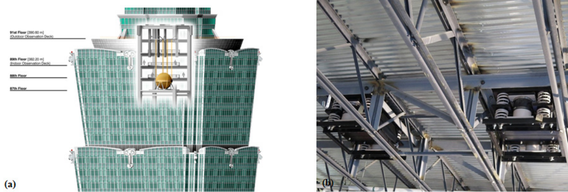
Fig. 1 Examples of TMD application: (a) Taipei 101; (b) Slab of education facility(DEICON)
