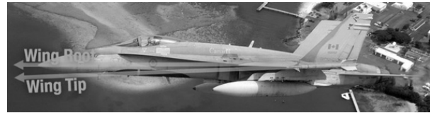
Fig. 2. Change of Incidence Angle on F-18
