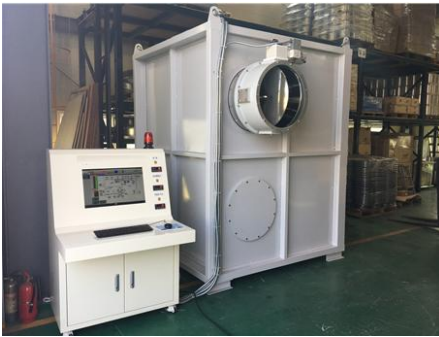
Fig. 8. Remote monitoring control test using test chamber and control panel
