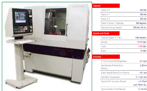
Fig. 3. FG350, Diamond turning machine & capacity.
