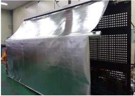
Fig. 1. The mockup of foldable safe pathway system[4]
