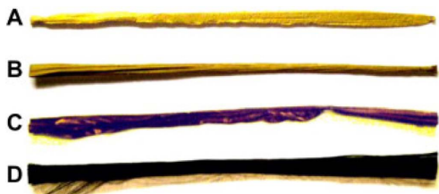
Fig. 8. Photograph images of stabilized flame retardant PAN composite electrospun nanofibers including CNT ochre under various temperatures and Oxi-PAN fiber; (a) 190°C, (b) 220°C, (c) 240°C, (d) Oxi-PAN fiber. Reproduced with permission [56]. Copyright 2013, Elsevier
