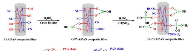
Fig. 5. Scheme of fabrication method for FR-PVA/PAN composite fiber. Reproduced with permission [43]. Copyright 2018, MDPI
