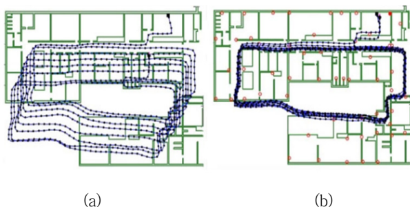
[Figure 1] Accumulated Errors in the PDR Technique (a) and Calibration Results (b)
