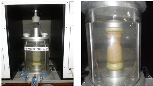
(e) Sample consolidation (f) Cyclic loading
