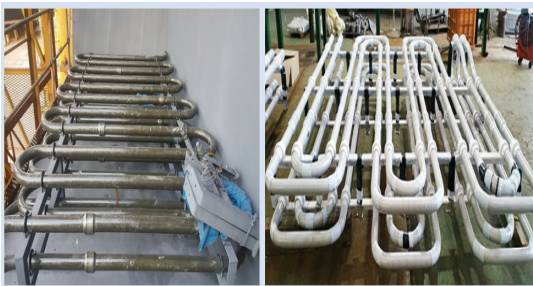
Fig. 6 Steam pipe in fuel tank
