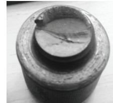
Fig. 2 Appearance of damaged high strength bolt
