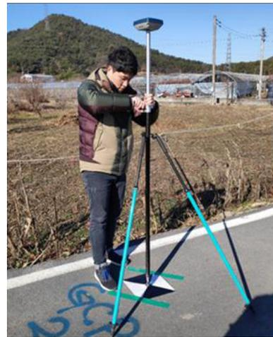
Fig. 4. GCPs and CPs surveying
