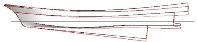
(a) Initial draft (black) and main draft (red) before viscous flow calculation set by potential flow analysis
